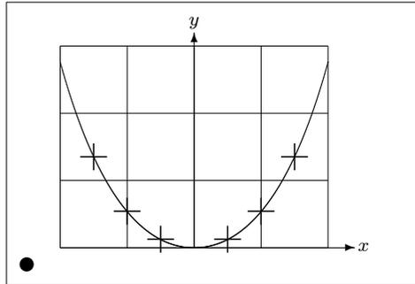
In this figure, each symmetric half of the catenary  $y = \cosh x - 1$  is approximated by a quadratic Bézier curve. The right half of the curve ends in the point  $(2, 2.7622)$ , the slope there having the value  $m = 3.6269$ . Using again equation (5.1), we can calculate the intermediate control points. They turn out to be  $(1.2384, 0)$  and  $(-1.2384, 0)$ . The crosses indicate points of the *real* catenary. The error is barely noticeable, being less than one percent.
